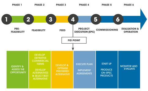
Figure 1: Phased Development of an Oil and Gas Industry Project
